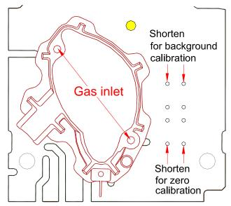
Figure 5 Part of the PCB with holes for gas inlets marked.
