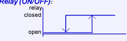
Figure 4 The relay output
