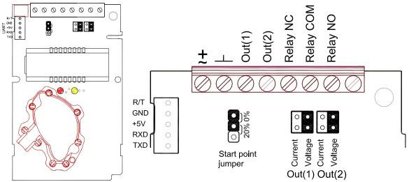
Figure 7 The aSENSE RL printed circuit board with CO<sub>2</sub> sensors for measuring ranges 0-3000ppm and 0-4%.
